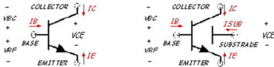
Figure 2. Current and Voltage Reference Arrow System
