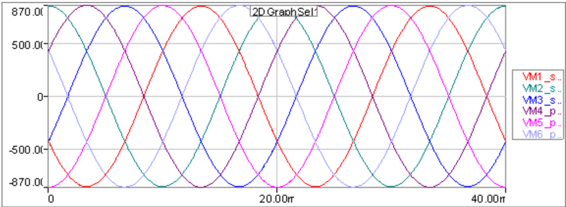
Figure 5. Simulation results – voltages on the primary and secondary sides of the transformer
